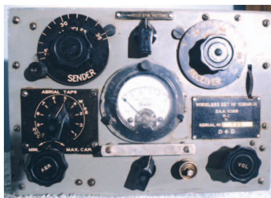
● Fig. 2: The WS No. 108 backpack set, again it has separate tuning dials for receiving and transmitting. The netting switch is at the top centre (see text).
