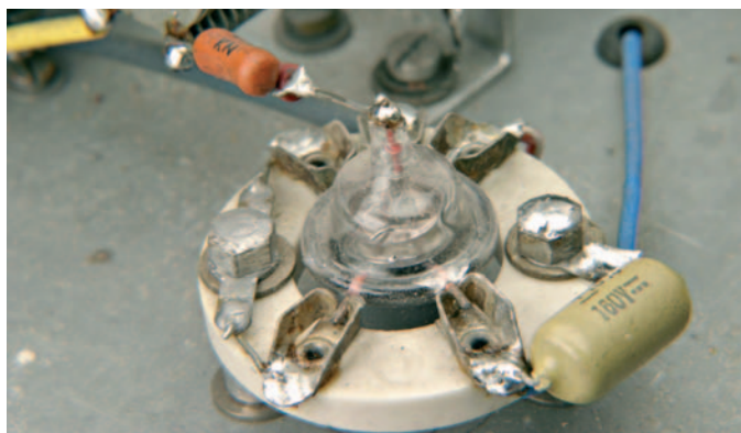
● The 954 acorn valve (originally designed specifically for v.h.f./u.h.f. operations) mounted on its special holder (see text).
