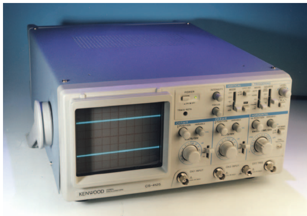
● Fig. 2: Another Kenwood 'scope! Readers may end up thinking that PW has a 'bias' towards Kenwood's oscilloscope range and in fact this is partly true as their range of instruments provide good value and reliability. This model is the CS-4125, one of the dual channel (double trace) instruments. Although more expensive than the basic 1305 and 1010, this 'scope offer two channel display and has a specification including a 20MHz bandwidth.
