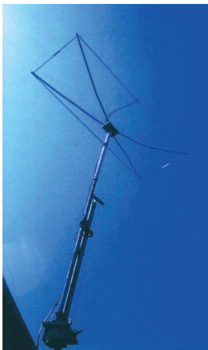
● Fig. 1: 50MHz Moxon Rectangle antenna at the QTH of Adrian Ball G8PSF. Based on the PW March 2004 construction article by Geoff Cottrell G3XGC.
