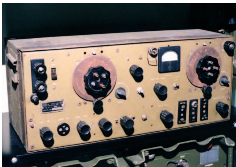
Fig. 1: The ZC1 MkI single band, no wavechange switch transmitter-receiver. Note the separate receiver (right) and transmitter tuning dials.
