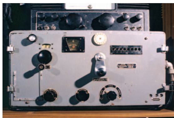
● Fig. 3: The German HMZL receiver, the large handle in the centre is the wavechange switch! The odd knob (top centre) is a later addition and will soon be removed.
