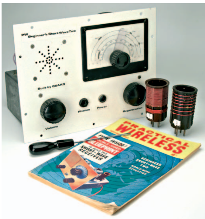
● The Beginner's Short Wave Two, as built by Richard Ayley G6AKG, from the original design (Richard spent several years collecting the more difficult-to-find components such as the Eddystone formers to build it as close as possible to the G3OGR design). See text for more details.
