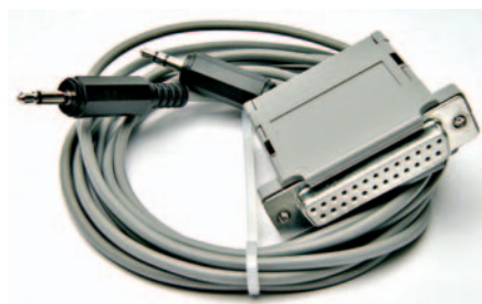
● Fig. 1: The receive-only Pervisell data-mode interface has an audio 'pass-through' lead to connect to the sound-card's input.
